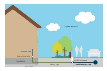
This diagram shows how a property is typically connected to the water mains from the communication pipe supplying fresh, clean water to the home. These pipes are usually owned and maintained by the local water company and each home then has its own supply pipe or common/shared supply pipe (serving multiple properties), which is owned and maintained by the property owner(s).
